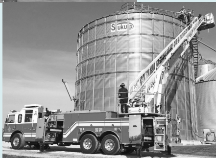
Left: This rig from the Batavia Fire Department was used as a pulley base during the grain bin rescue drill. The ladder can extend up to 100 ft and the basket at the end can carry over 500 lbs. Rigs like this one are used by fire departments to perform high angle rescues.
